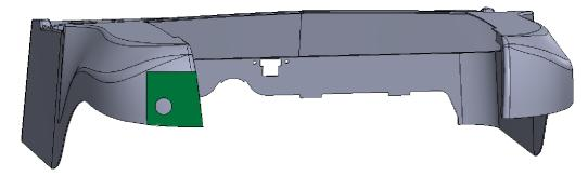
PLACE TEMPLATE ON CORNER OF BODY AS SHOWN. CUT HOLE IN BODY BEFORE PLACING ON CAR. FLIP TEMPLATE FOR USE ON OPPOSITE SIDE.
